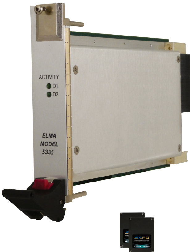
Dual drives in one 3U VPX slot
